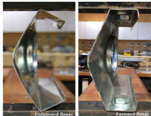
Fig -2: Web Crippling Failure
